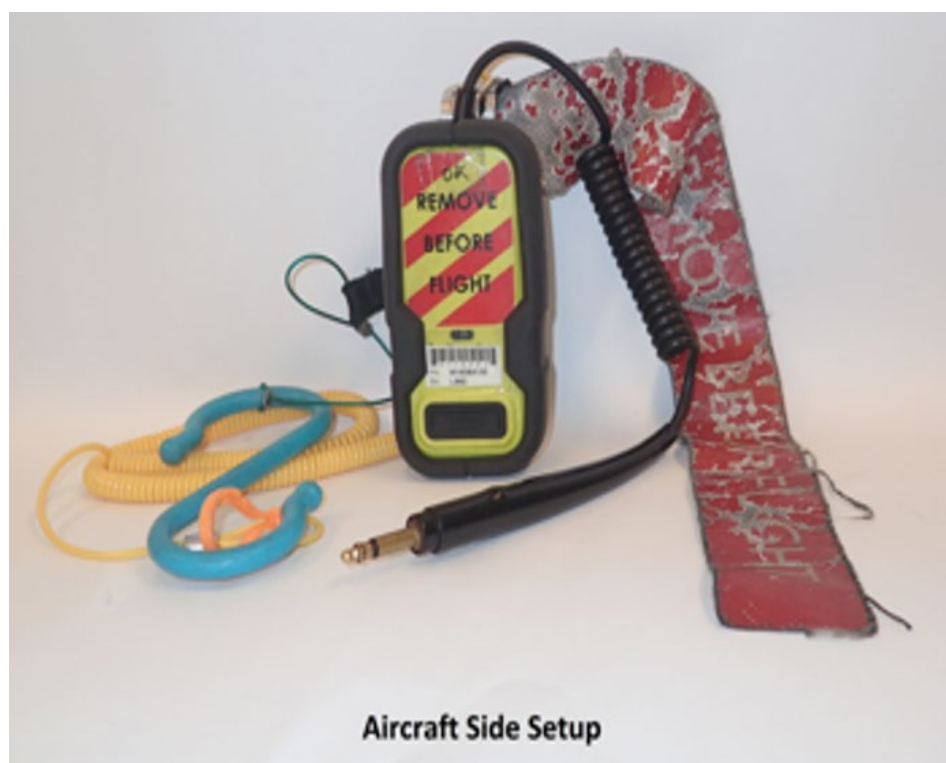
Photo 3: Wireless Headset Setup for Aircraft Side
